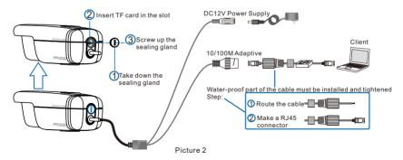
[Note]: Some models support PoE (Power on Ethernet). Only have to connect RJ45 connector to PoE switch and no other power supply is needed.
