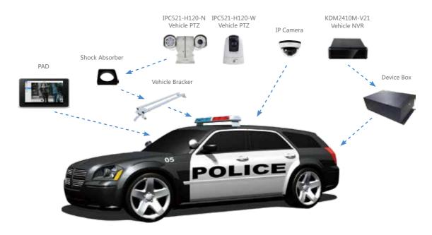
The embedded communication functions within the KVMS works through 3G/4G and wireless network while audiovisual data is uploaded to command center and shared with users within the same networking group. The KEDACOM KWTP wireless protocol used by our system ensures very low latency and drastically reduces packet loss for video streaming while delivering superior image quality.
