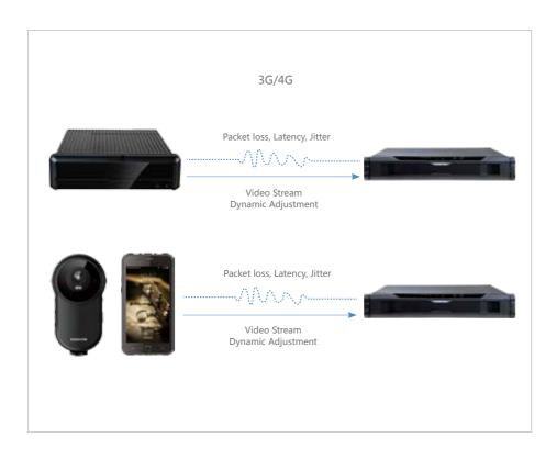
Vehicle and Portable Mobile peripheral units can be connected to KDM2800 series VMS directly without any extra gateway equipment. It can also support the KEDACOM Wireless Transmission Protocol (KWTP) which can adjust video streaming strategy based on real-time network status monitoring and ensure a continuous and reliable transmission to VMS over 3G/4G and wireless network.
