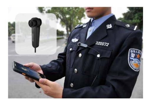
USBCAM-100 is an external USB camera which can be used together with IPW200 and DSJ-U1. It can be disguised as a button and used for covert surveillance. It weighs just 30 grams which is conveniently worn with service uniforms.
