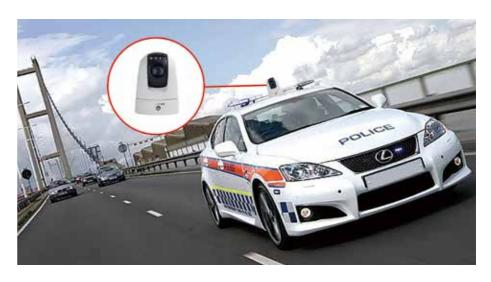
The KEDACOM Vehicle Mobile System (KVMS) supports wireless connectivity between vehicle-mounted camera and mobile NVR. It also support 9V~36V broad range voltage input suitable for both 12V and 24V in-vehicle power supply which can feed power to the cameras. The fixed cameras have an embedded microphone which makes wireless communication simpler. The installation of the KVMS saves time considerably and is cost effective.
