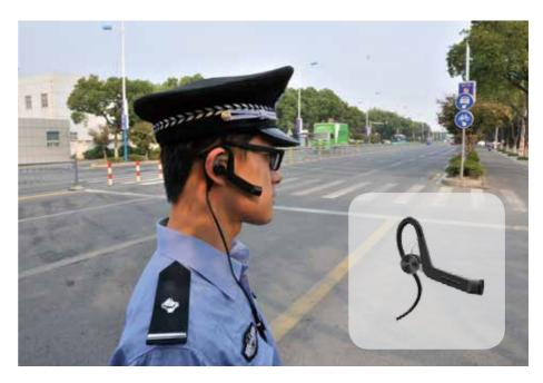
USBCAM-200 is an ear-hook camera which can be used together with IPW200 and DSJ-U1. On first glance, It looks like a Bluetooth headset from appearance but it enables true covert surveillance. USBCAM-200 also has a lens with F2.2 large aperture and diagonal Field of View (FOV) up to 100°, to acquire videos at 720p@30fps. The built-in microphone and headset can be used for communication with command center in intercom mode.
