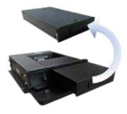
KDM2410M-V1 possesses a 2.5-inch hard disk drawer, which can be locked and supports 4TB storage. A structure comprising of a spring capsule with double shock-proof design, protects hard disk while the vehicle is being driven on bumpy roads. Besides, the drawer design helps users change hard disk more conveniently. With the help of USB interface in its rear panel, the audiovisual records can be retrieved quickly.
