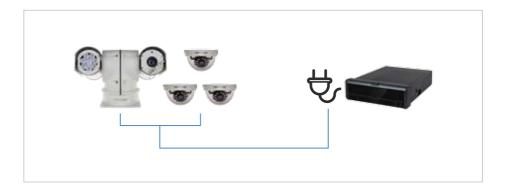
Cameras are connected to KDM2410M-V21 either through its combined aviation plug or embedded WiFi. A stable physical connection is assured with an aviation plug even when vehicle is being driven on bumpy roads. The combined aviation plug not only supports Ethernet and analog cameras' interfaces, but it can also feed power backward to all cameras, which makes the installation more conveniently.
